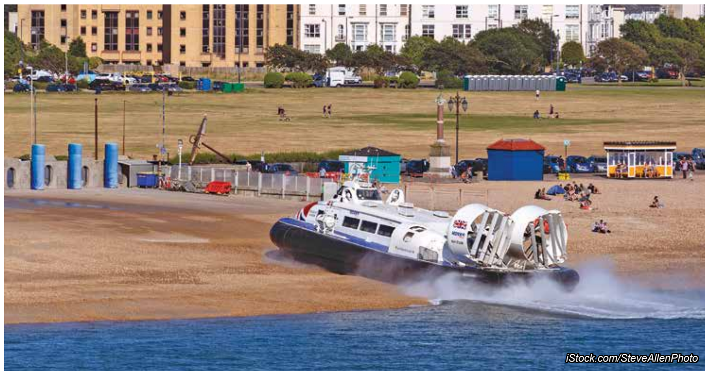
Hovercraft are far more flexible than traditional ferries in terms of docking as well as the water depth over which they can operate. This may allow passenger service to areas with shallower water, such as parts of the South Bay and the Delta.
