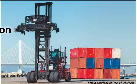
The Port of Oakland is embarking on a goal to achieve emission-free cargo operations. Zeroemission cargo operations would require most port trucks and terminal equipment be powered by sources other than diesel fuel.
