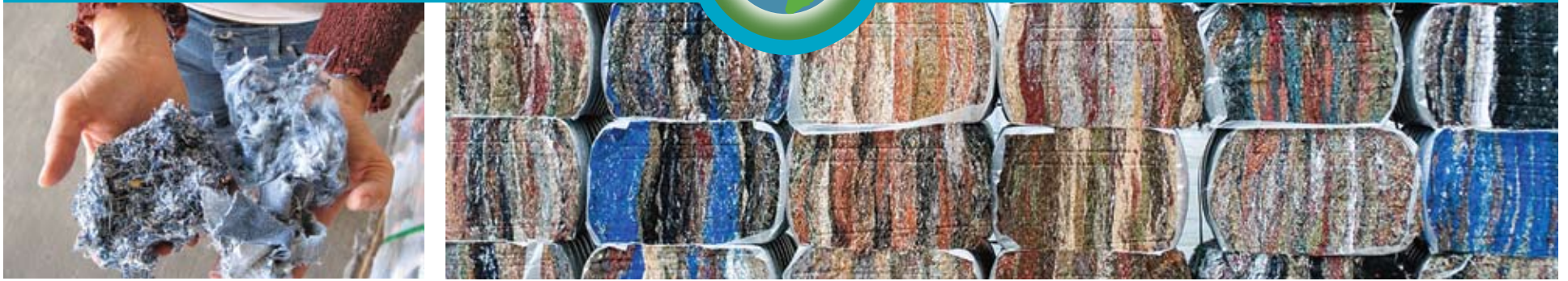
Old items that are collected but can't be sold are shredded and used in 'shoddy cloth,' which is used for carpet padding, insulation, sound-proofing material (like the example below) and all sorts of other things.
