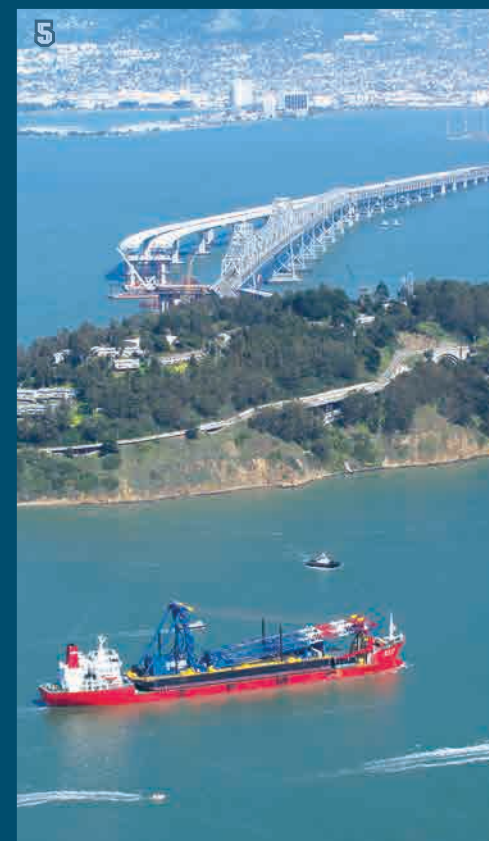
The “Left Coast Lifter” crane and barge slipped under the Golden Gate, skirted the San Francisco shoreline and passed under the West Span of the Bay Bridge; the final destination is the Bay Bridge East Span construction zone on far side of Yerba Buena Island (visible in image 5). Photos 1 and 2 are by Noah Berger and the aerial photos 3, 4 and 5 are © 2009 Barrie Rokeach.
