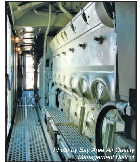
Locomotive 2015's engine was upgraded to minimize diesel emissions and increase fuel efficiency.
