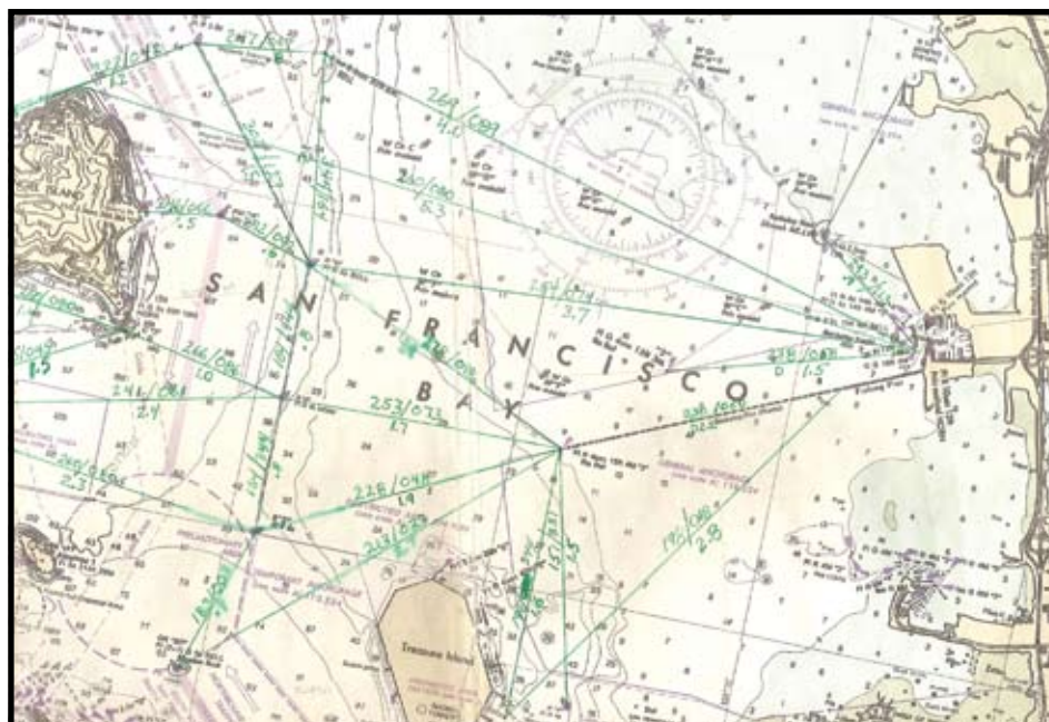
Notes made on navigation charts can be used to plot courses and distances between frequently used locations when “buoy hopping.”
