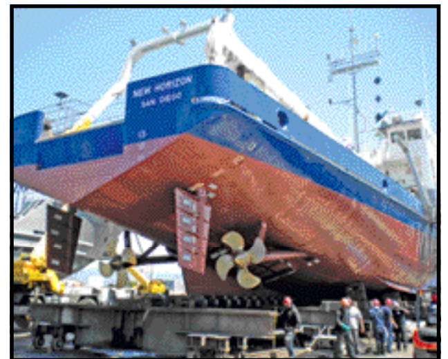
Completing underwater hull and machinery repairs on Scripps Institution of Oceanography’s “R/V New Horizon” at Bay Ship & Yacht’s shipyard in Alameda, CA.
