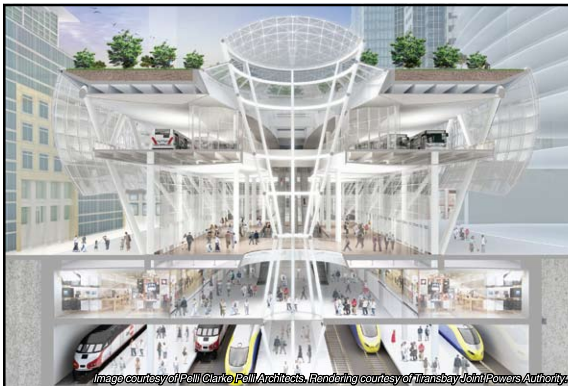
Image courtesy of Pelli Clarke Pelli Architects. Rendering courtesy of Transbay Joint Powers Authority. This cross section of the new terminal shows the bus deck on the top level and the underground train station serving both Caltrain and the California High-Speed Rail system.
