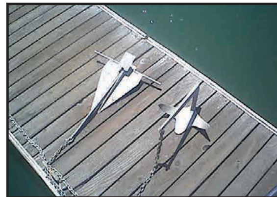
Danforth anchor on the left and a Bruce anchor on the right.
