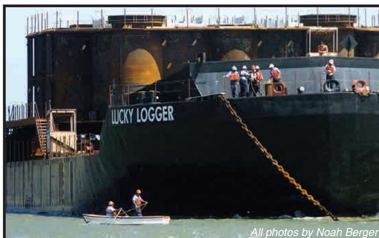
Perched on the deck of the Lucky Logger barge, the East Span footing box makes its way through the Panama Canal.
